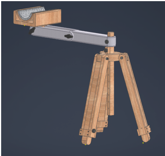
Figure 1: The Supporter at its lowest height and linkage fully extended.
